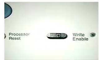
Access Level 3 – The Slide Switch is to the Right
