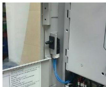
Door Switch in Access Level 2
