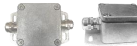
FP-09512 2way and EOL Junction Boxes with strain relief cable glands and 1x EOL for monitoring. (Obsolete)
