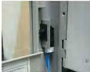
Door Switch in Access Level 1
