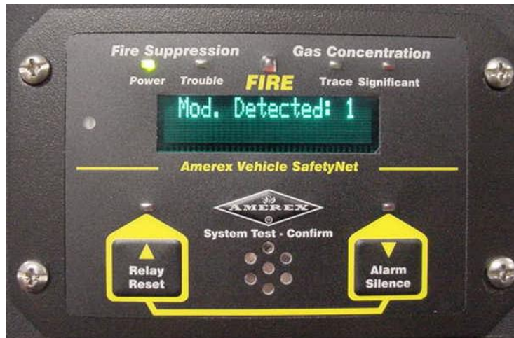
Figure 26- SafetyNet recognizes new Module in the Configuration,
