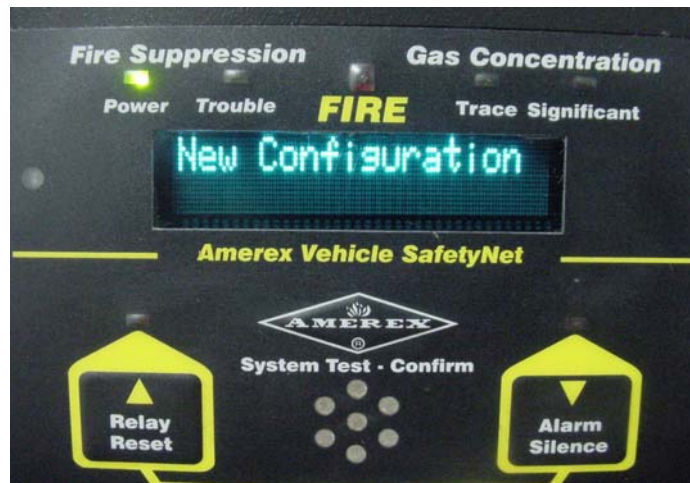
Figure 17 - The SafetyNet system acknowledges the New Configuration
