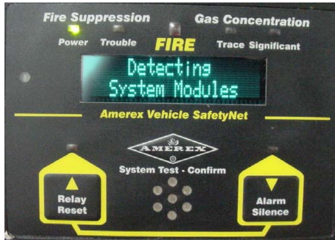
Figure 18 - SafetyNet verifies the Software Configuration matches the Hardware Configuration
