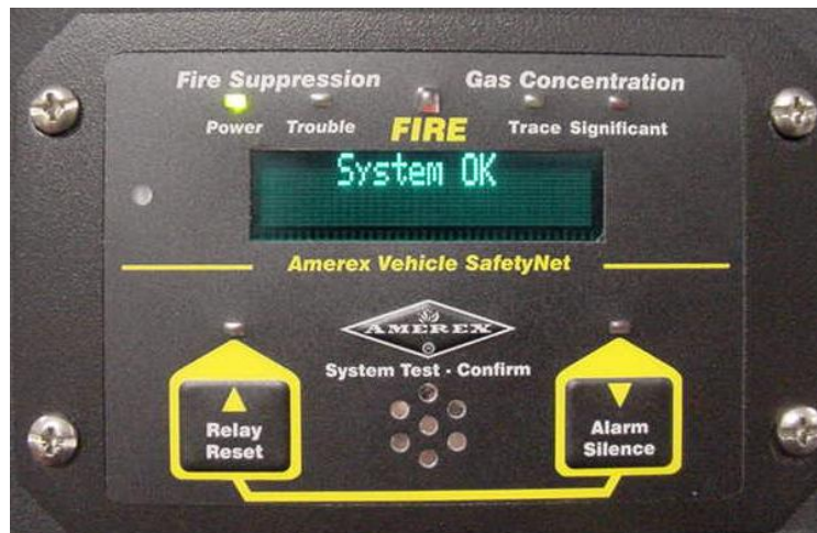
Figure 6 - The Operator Display has established Communication with the module
