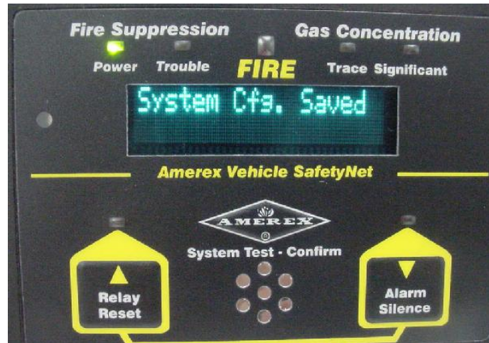
Figure 9 - After pressing the System Test - Confirm button, the SafetyNet System "memorizes" the new configuration
