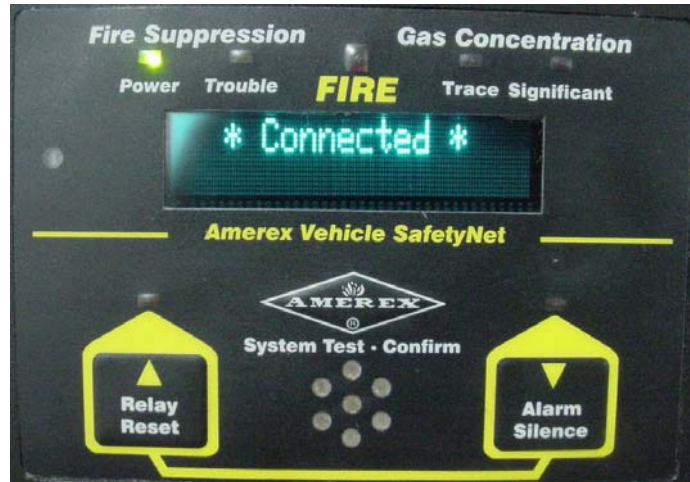
Figure 23 - When uploading a new Configuration, your PC connects to the SafetyNet system,
