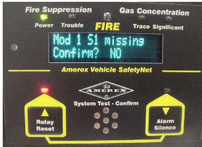
Figure 7 - The system has recognized that Sensor #1 is missing ( by design in this example )
