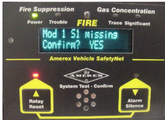
Figure 8 - Press either the Relay Reset or Alarm Silence buttons to toggle the screen to "Yes". Press the System Test – Confirm button to acknowledge that you recognize that sensor #1 is missing by design
