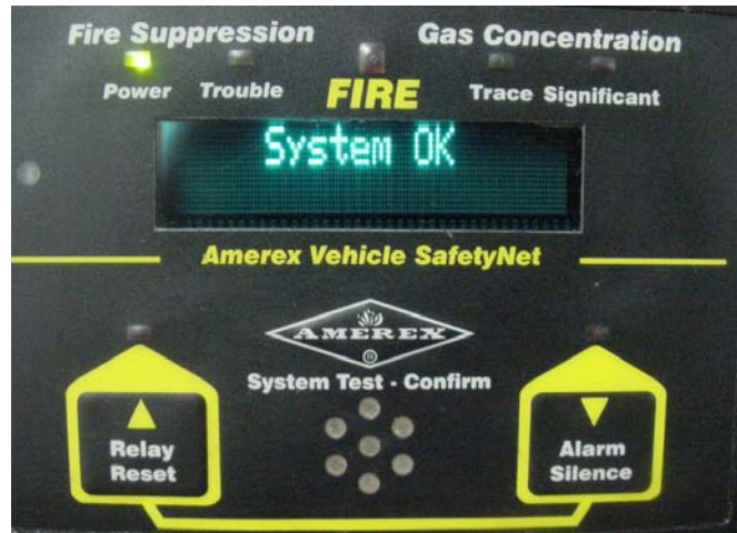
Figure 20 - SafetyNet verifies that the Software and Hardware match
