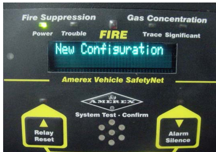
Figure 24 - The SafetyNet system acknowledges the New Configuration,
