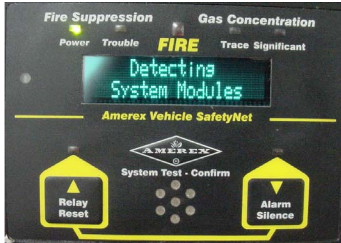
Figure 25 - SafetyNet verifies the Software Configuration matches the Hardware Configuration,
