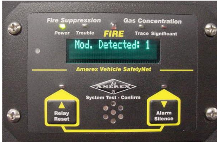
Figure 5 - Only (1) module has been detected
