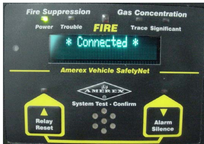
Figure 16 - When uploading a new Configuration, your PC connects to the SafetyNet system
