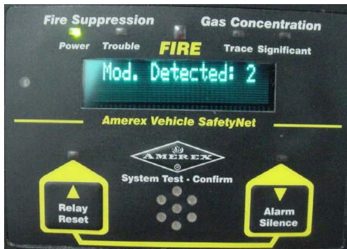
Figure 19- SafetyNet recognizes the two Modules in the Configuration
