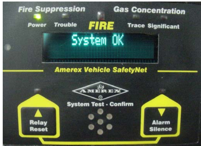
Figure 27 - SafetyNet verifies that the Software and Hardware match,
