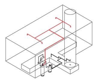
"IS" has the first UL Listing allowing nozzles to be placed up to 23'-4" above the floor – now you can protect large vehicle paint spray booths that are used for trucks and heavy equipment with a fully UL Listed system that has been specifically tested using live fires for this application.
