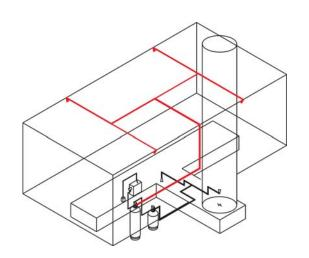
"Standard-sized Down Draft" Booths using the ceiling as a plenum – The Amerex "IS" system has unique UL Listings that allow for options regarding the placement of nozzles. Nozzles may be placed in the traditional "H" pattern or they may be placed "Inline" down the center of the ceiling or even at the side walls. This allows nozzles to be placed out of the way for periodic replacement of the filters saving you time, money and hassle.
