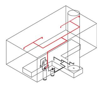
Nozzles may be placed down the center of a standard sized booth to make filter replacement easy.
