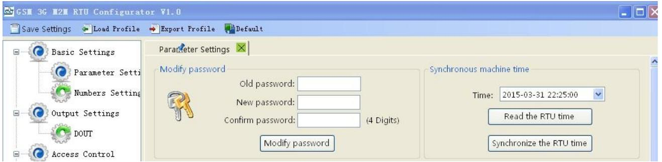
**Save Settings:** Click it to save all of the PC Configurator parameters to the RTU;
