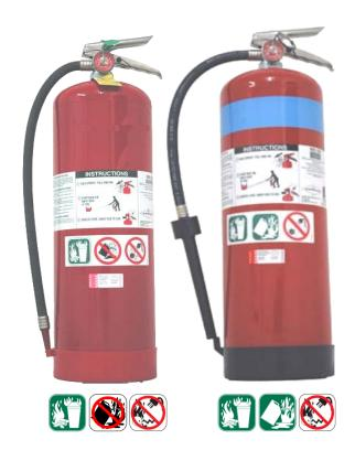
**Model 240** utilises the cooling, soaking and penetrating effect of a 13-17m stream of WATER. The 60 sec. discharge time makes it very effective for inexperienced operators to use on Class A fires. Protect from Freezing by adding the Model 506 Stream/Anti-Freeze charge. In Western Australia, South Australia and other areas with a high level of chloride content water it must be corrosion protected by adding the Model 507 charge.
