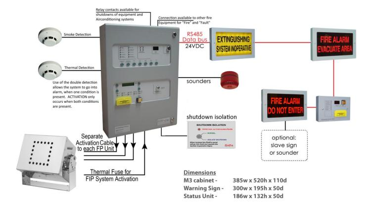
**SIGMA XT Panel is the only FIP that is currently approved BY FirePro**, this panel and ancillary equipment will properly monitor the FirePro aerosol generators in accordance with the requirements of AS 4487. The Sigma XT series can be used as a main FIP or slave panel from other FIP manufacturers.
