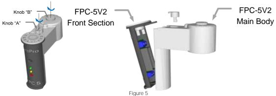
Step 2: Pass the Condensed Aerosol Generator wires through the FPC-5V2 main body. It is important to pass the Condensed Aerosol Generator wires from the same opening of the adaptor plate/junction box coupling.
