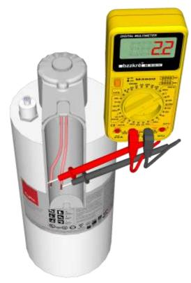
Figure 17: Measuring the Condensed Aerosol Generator's resistance
