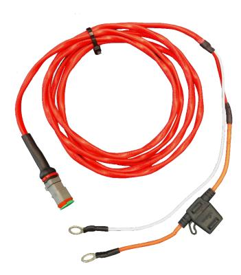
The Battery Lead is designed to connect directly to Battery Terminals – using M10 uninsulated ring terminals.
